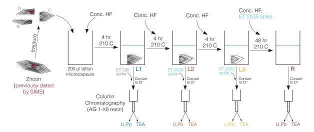
**Figure 1.** Schematic illustration of the step leaching methodology employed in this study. U, Pb fractions separated by column chromatography for each leachate of each zircon fragment were analyzed on an IsotopX Phoenix 62 Thermal Ionization Mass Spectrometer, while TEA solutions were analyzed for trace element concentration on a Thermo Element 2 ICPMS at Princeton University.
