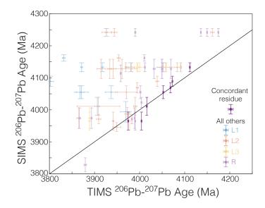
**Figure 5.** Two-variable cross plot of SIMS spot ages and TIMS <sup>207</sup>Pb/<sup>206</sup>Pb ages for each fragment and leachate. Concordant residues (bold) plot along the 1:1 line, while others plot above. Horizontal data arrays result from one SIMS spot age per grain plotted against up to four TIMS ages per fragment, with multiple fragments per grain.
