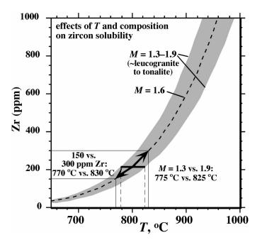
Figure 1. Solubility of zircon as function of temperature, *T*, and melt composition, *M*. Large variation in *M* results in relatively small change in solubility; thus, large uncertainty in melt-phase composition introduces small error in estimated temperature (tonalite vs. leucogranite, 50 °C). Likewise, because zircon solubility is so strongly temperature dependent, large errors in estimated *Z* r concentration in melt introduce small errors in temperature estimate.
