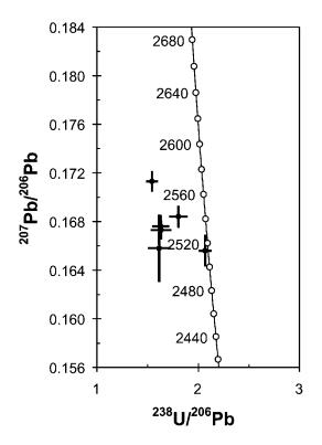
**Figure 6.** Tera-Wasserburg ( $^{207}$ Pb/ $^{206}$ Pb vs.  $^{238}$ U/ $^{206}$ Pb) diagram for zircons extracted from sample Ch Zr 4. Data points are plotted as 1 $\sigma$  error crosses.
