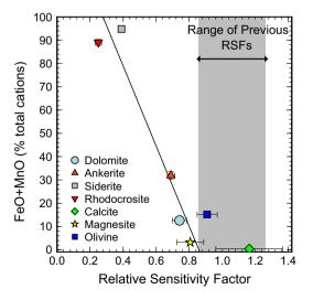
Fig. 4. Plot showing the correlation between the RSF<sub>Mn/Cr</sub> measured by ion implanting and the FeO + MnO percentage of the carbonates. The line corresponds to a weighted regression through the carbonate points. Error bars are plotted for all points in both x and y but, in some cases, are smaller than the symbols.
