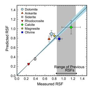
Fig. 8. Figure showing the correlation of the measured RSF versus the predicted RSF from Eq. (7). These data show good correlation close to unity with a slope of  $0.97 \pm 0.06$ .
