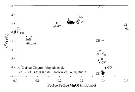
**Figure 3.** A plot of the  $\Delta^{17}$ O versus  $\text{FeO}_x/(\text{FeO}_x + \text{MgO})$  ratio for samples of bulk chondrites gives even better resolution of the chondrite groups than do the chemical parameters plotted in Figure 1 or the  $\delta^{17}$ O- $\delta^{18}$ O distribution in Figure 2.
