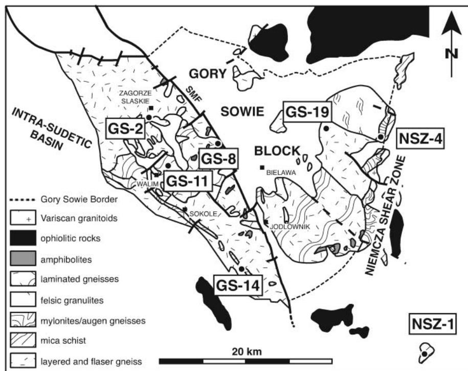
**Fig. 3.** Simplified geological map of the Góry Sowie Block and Niemcza shear zone. The map shows the main lithological units, structural elements and sample locations (modified after Bröcker *et al.* 1998). SMF, Sudetic Marginal fault.
