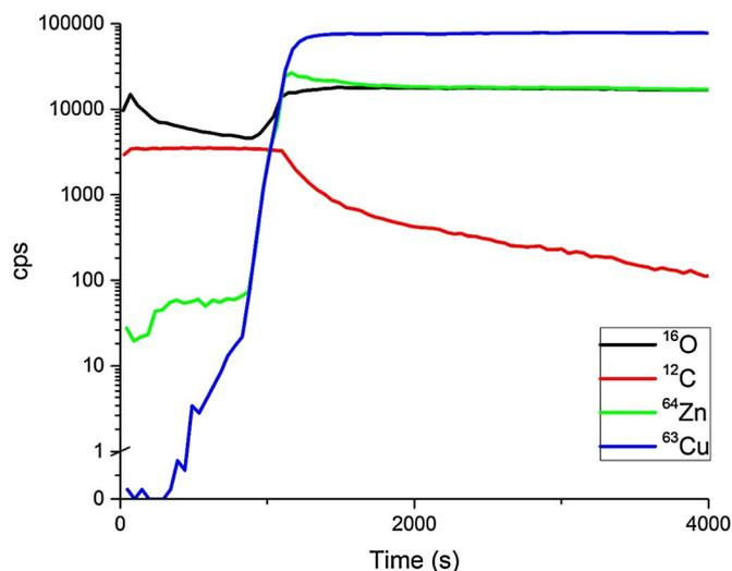
**Fig. 1.** Depth profile of unaged coating 1 on a brass substrate. The counts per second from four isotopes were analysed during a 4000 s measurement.
