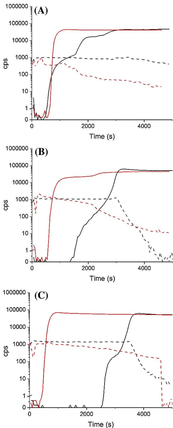
Fig. 2. Copper (solid line) and carbon (dotted line) depth profiles of coating 1 (black) and coating 2 (red) artificially aged (A) 72, (B) 240 and (B) 720 h. (For interpretation of the references to colour in this figure legend, the reader is referred to the web version of this article.)
