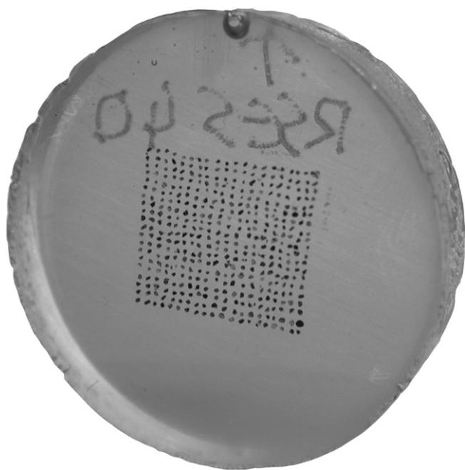
**Fig. 7.** Zircons mounted in a  $20 \times 20$  grid pattern. The “way-up” registration arrow on the back of the mount allows each grain to be identified and extracted for further analysis.
