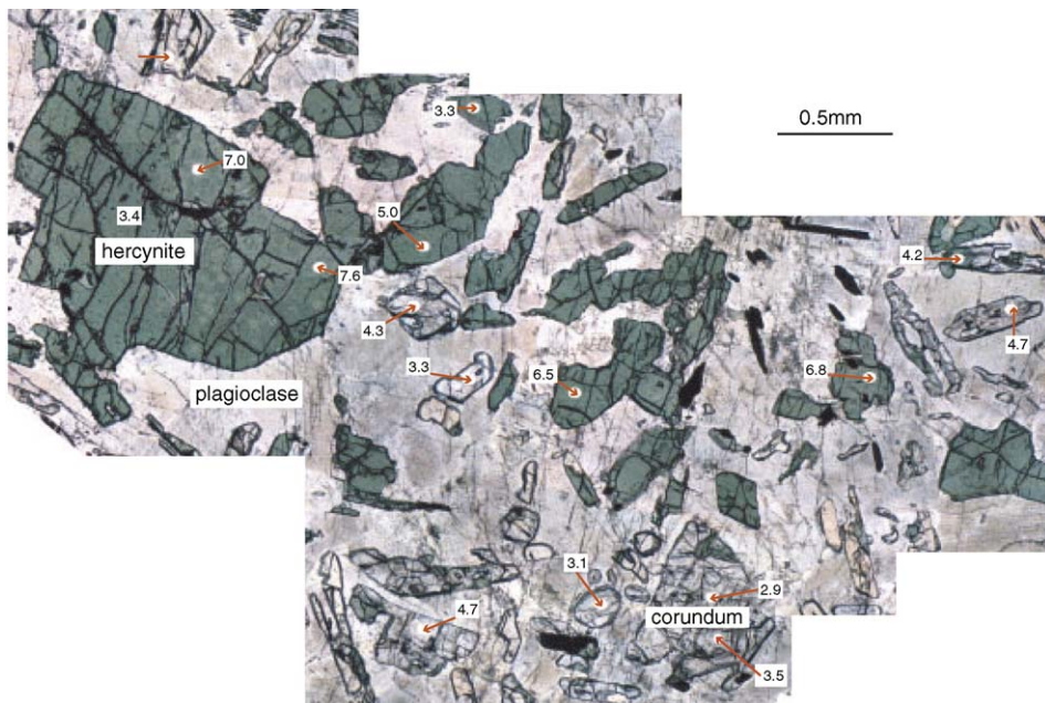
Fig. 5. Photomicrograph showing ion microprobe sites and distribution of \delta^{18}\text{O} values in sample VB492-1005.0 from the south Eastern Deeps zone of the Voisey's Bay Intrusion. All \delta^{18}\text{O} values are in per mil relative to VSMOW.
