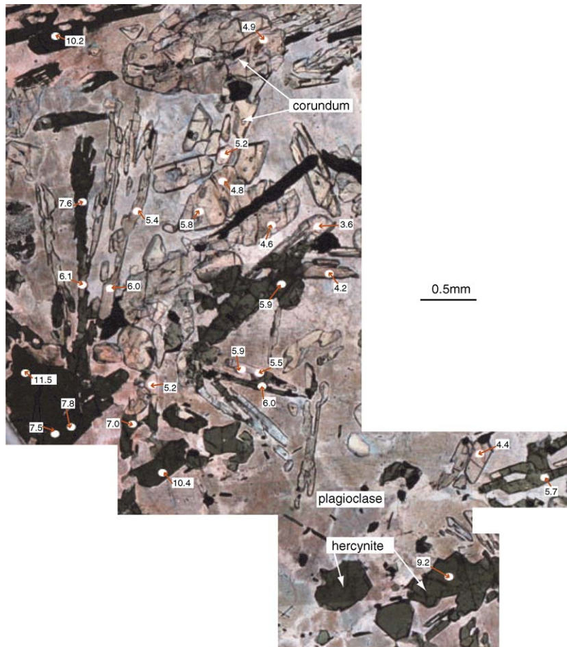
Fig. 6. Photomicrograph showing ion microprobe sites and distribution of \delta^{18}\text{O} values in sample VB523–762.0 from the Eastern Deeps zone of the Viosey's Bay Intrusion. All \delta^{18}\text{O} values are in per mil relative to VSMOW.
