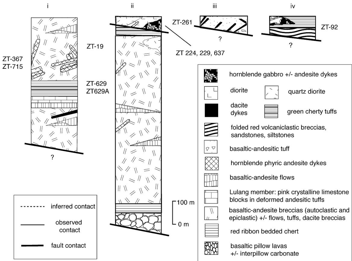
Fig. 3. Schematic stratigraphic sections illustrating the age and relationships of volcanic and intrusive units within the Zedong terrane and samples analyzed herein. The locations of i–iv are shown in Fig. 2.
