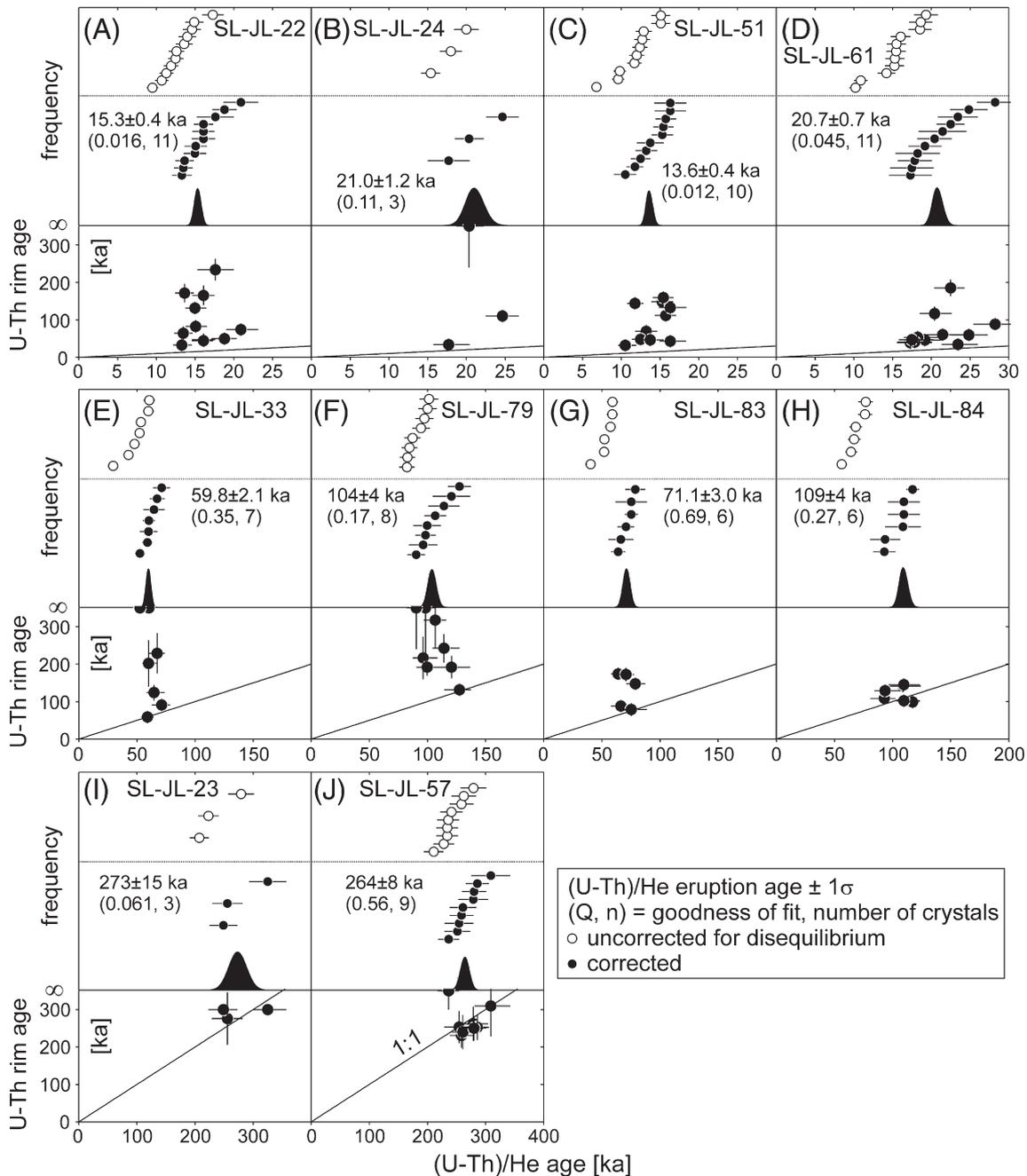
**Fig. 2.** Combined U-Th and (U-Th)/He zircon ages. Each panel shows the uncorrected ages (top), the disequilibrium-corrected ages, and a Gaussian fit to replicate analyses representing the modeled eruption age (middle). The lower panel compares corrected (U-Th)/He ages with the U-Th zircon rim crystallization ages. Ages below the 1:1 line are impossible because zircon crystallization must predate the eruption.
