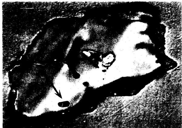
Fig. 4. Transmitted light photomicrograph of Orgueil olivine grain 2–28, which has been mounted in epoxy and polished. The maximum grain diameter is \sim 250 \mu\text{m} . The photograph was taken before oxygen isotopic analysis and is focused below the polished surface of the grain at a level where a glass inclusion with shrinkage bubble is visible near the bottom edge of the grain (marked by an arrow). McSween (1977) used similar features in isolated grains from other carbonaceous chondrites to argue that the isolated grains formed in chondrules.
