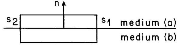
FIG. 2. The location of vanishing volume across the discontinuity surface in computing energy flux.
